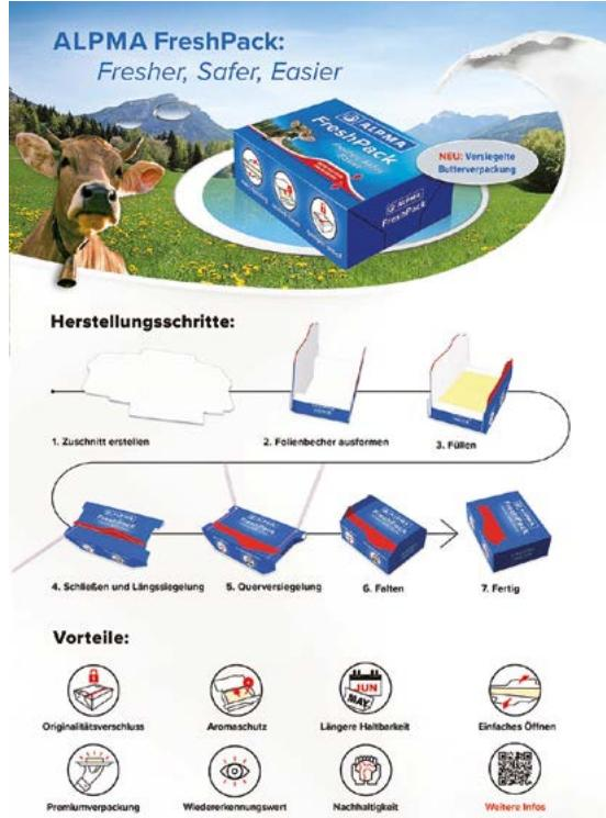
The ALPMA freshness packaging is folding packaging whose packaging film is continuously sealed on the closure side. Very special, innovative film cutting can be used to fold the film so that sealing zones occur outside of the product area. As a result of this, fresh butter aroma is verifiably kept in the packaging for longer and the shelf life is extended.
